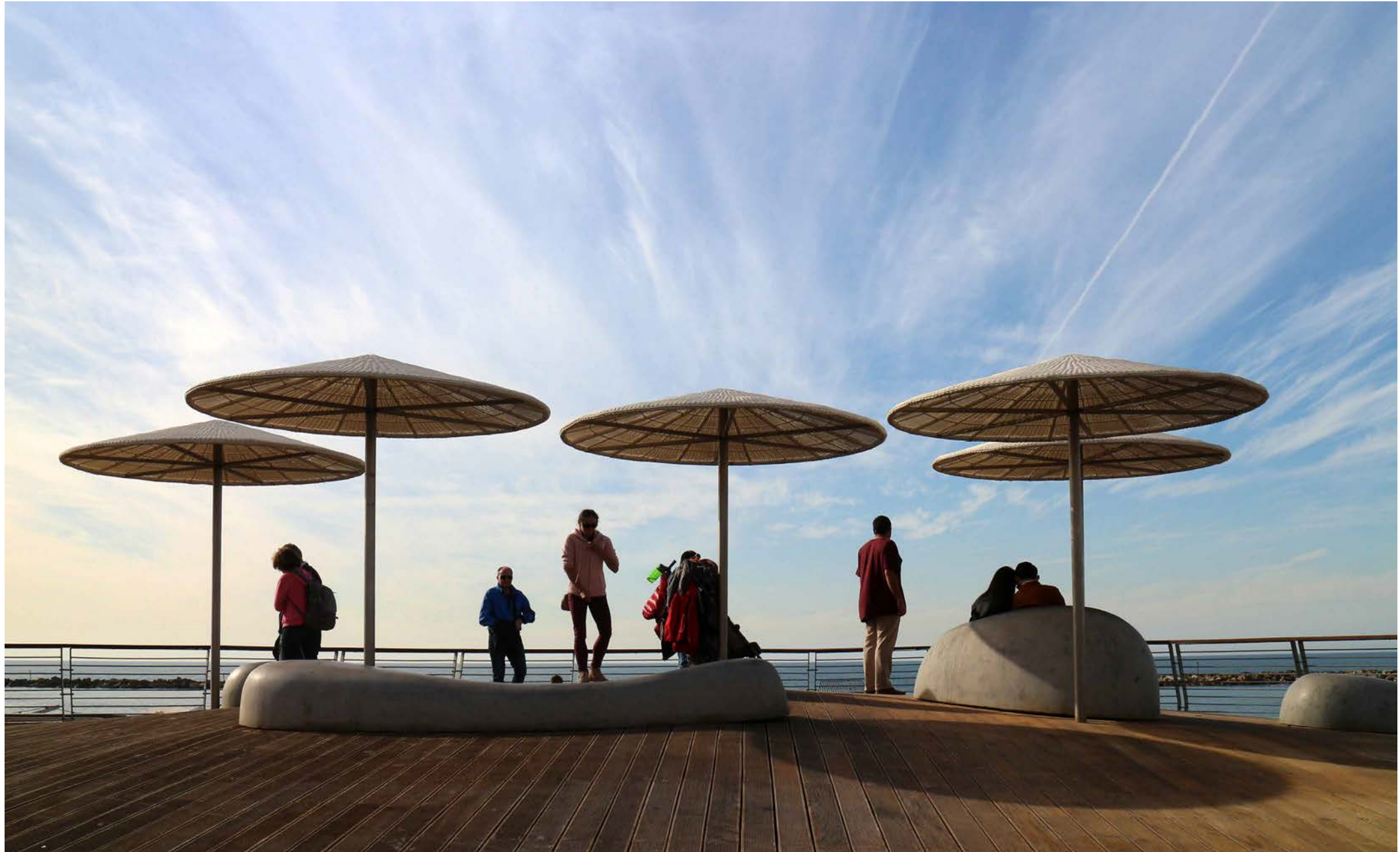
Specially crafted handwoven rattan parasols, along with seating pebbles cast in GRC, provide sitting and shade to the new urban terraces, constructed on the existing cafes rooftops.
